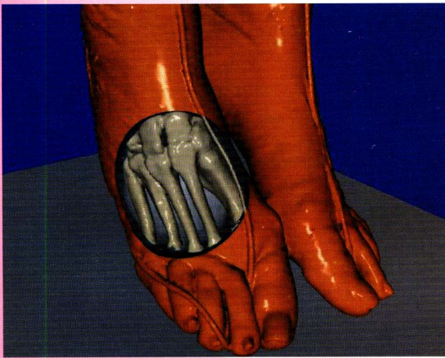
Figure 1. Complex visualization combining clipping, cutting, and volume rendering to produce a tissue lens, a special type of information lens.
