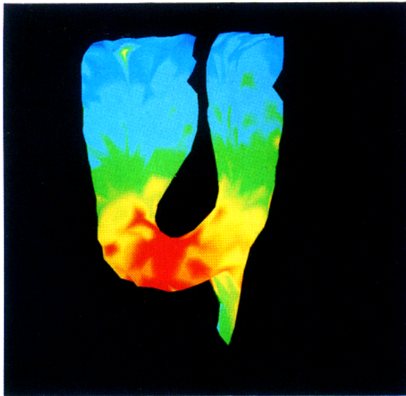
Figure 11 The GDM has its vertices colored based upon the generation which the vertex was created. This illustrates that model points are only added in the regions of the model still expanding.
