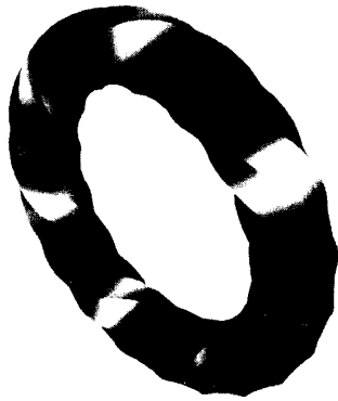
Figure 4: Stream polygon swept along closed path with uniform rotation.
