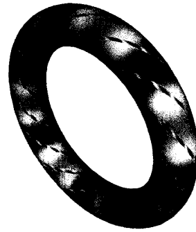
Figure 5: Streamtube with n = 49 sides. Every seventh side is colored with a different scalar data.
